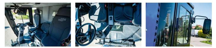
The cabin is equipped with **high-quality sound-proofing and vibration damping**. This allows the driver to focus even more effectively and perform their tasks efficiently and safely. The powerful thermal management system also ensures the best possible interior climate while working. The angle of the steering column can be adjusted and the cab can optionally be equipped with three seats.
