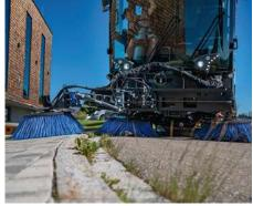
With the optional third brush, the span swept can be as wide as 139.8 in. This allows a larger area to be covered as well as sweeping on two levels.
